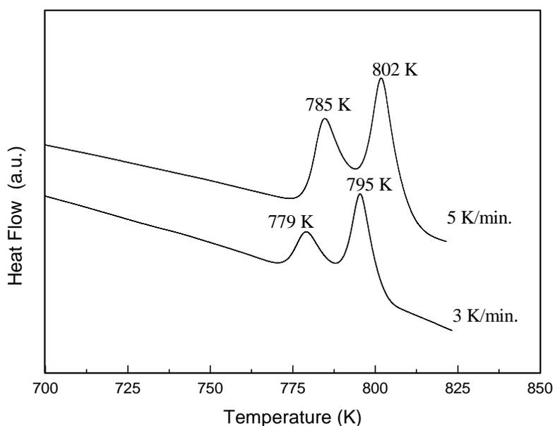
Fig.1. DSC curves of the amorphous 2605S3A alloy at two heating rates.
