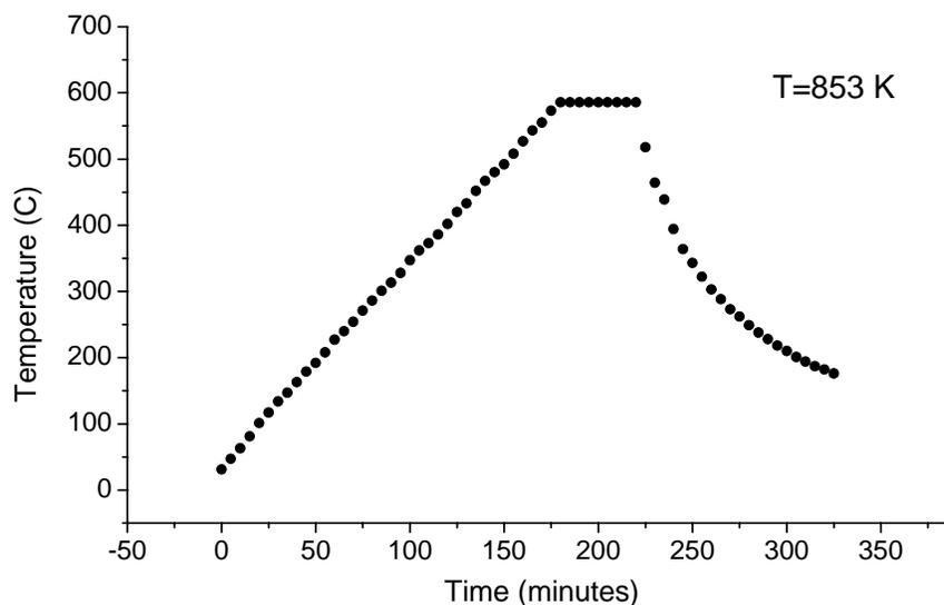
Fig.2. Typical heating and cooling treatment subjected to the alloy at CHR of 3 K/min.
