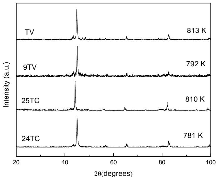
Fig.5. XRD patterns of the amorphous 2605S3A alloy after some of the heat treatments as indicated in the text.
