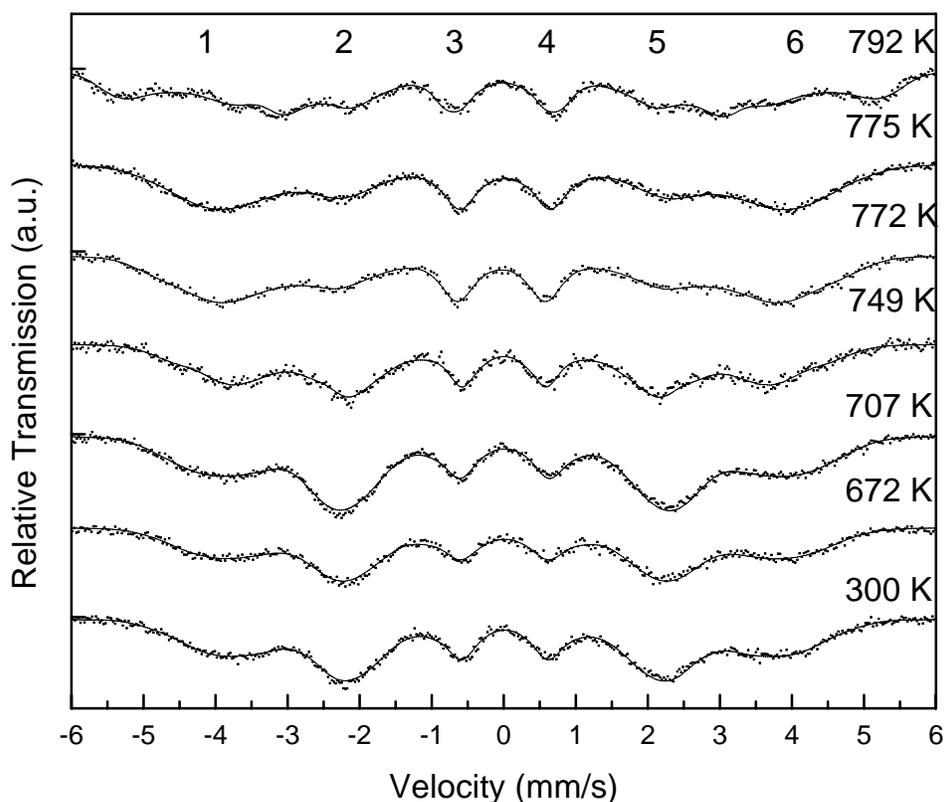
Fig.6. Mössbauer spectra of the amorphous and crystalline 2605S3A alloy annealed at different temperatures.
