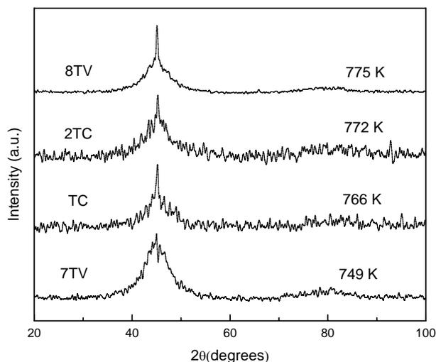
Fig.4. XRD patterns of the amorphous 2605S3A alloy after some heat treatments as indicated in the text.
