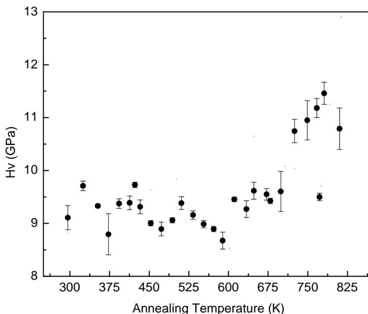
Fig.3. Vickers micro-hardness numbers variations from the amorphous 2605S3A alloy with different annealing temperatures.
