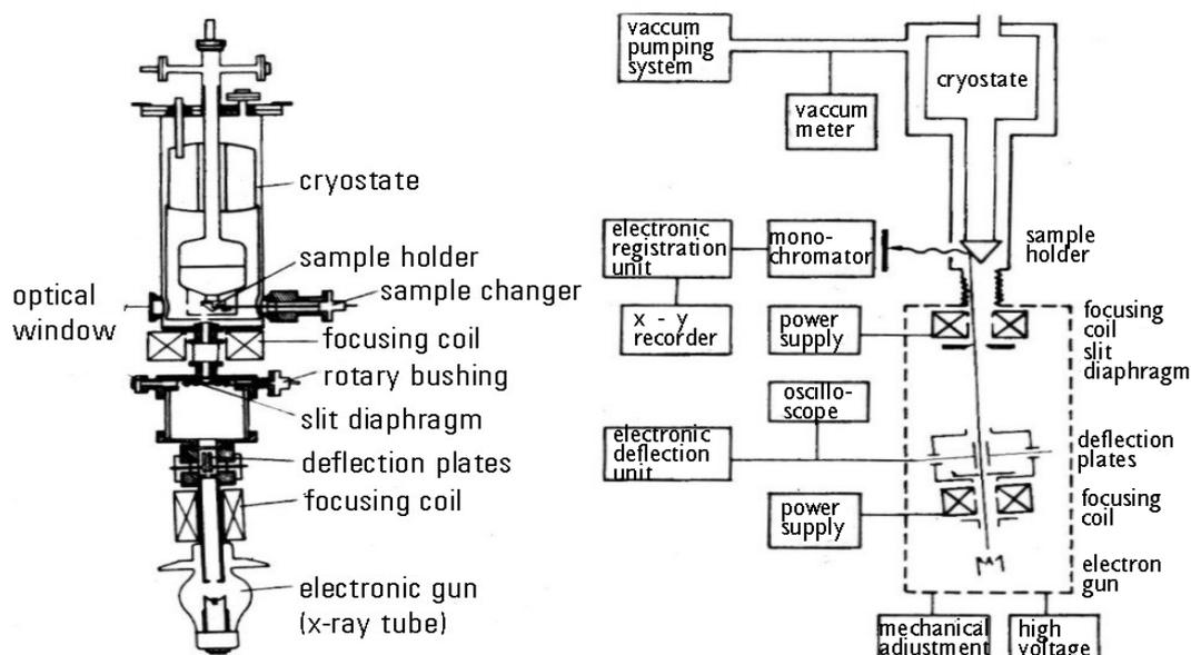
Fig. 3: Cathodoluminescence equipment, and schematic diagram of the involved components. The cathode of a common X-ray tube was adapted to the cryostat as electron-beam generator
