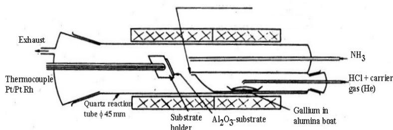
**Fig. 2:** Schematic apparatus design for the growth of epitaxial GaN films on ruby. The formation of GaCl at 850°C, and the epitaxial growth at 1000°C is enabled by a two-zone resistance-heated furnace.
