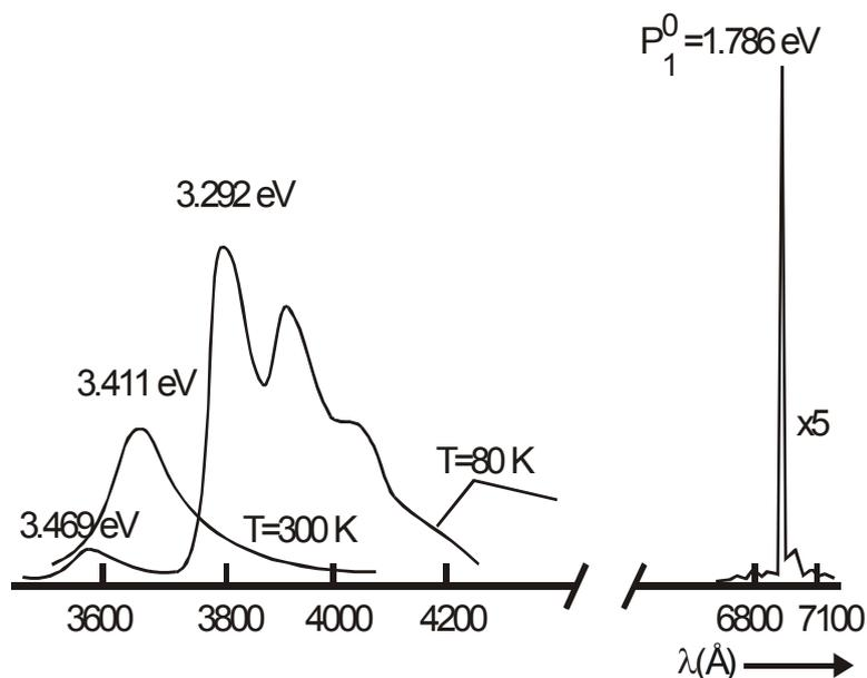
**Fig. 4:** Measured luminescence intensity vs. emission wave length of the specimen GaN/Al<sub>2</sub>O<sub>3</sub>:Cr at 80 K and 300 K, excited by a pulsed 30 keV electron beam on the GaN-layer side.
