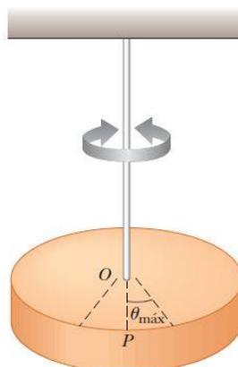
Fig. 4 General form of a torsional pendulum
