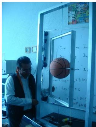
Fig. 8 Basketball inside the torsional pendulum system
