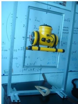
Fig. 9 Mini submarine inside the torsional pendulum
