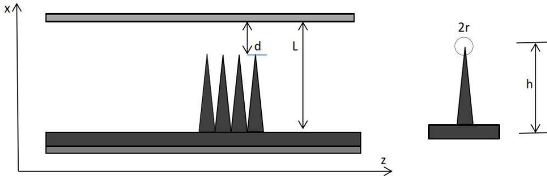
Fig. 1: Cold cathode emitter structure with nanoscale emitter tip (*right*). The cathode-anode distance is  $L$ , the distance of the emitter tip to the anode is  $d$ . The height  $h$  and the tip radius  $r$  of the cone result in an aspect ratio  $\sigma=h/2r$ . The applied voltage  $U$  generates a (global) electric field of about  $F=U/L$ , given that usually  $L \gg d$ .
