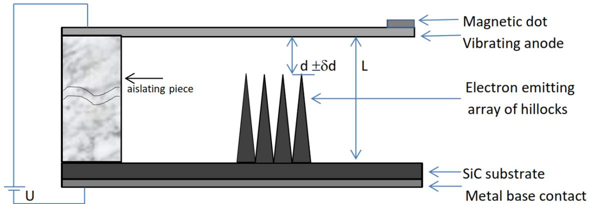
Fig. 4: Cold cathode emitter device, where the distance  $d$  between the tip of the emitter and the anode is allowed to oscillate by  $\pm\delta d$ . This may be achieved by a flexible substrate or a magnetically displaced anode.
